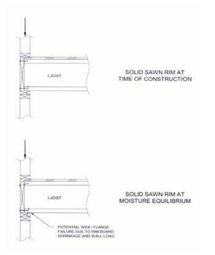
For lateral load transfer, the design limitation is often nailing from the sheathing into the rim. This nailing is required to develop and transfer shear forces in the diaphragm to the wall or foundation below. A rim board that is short will significantly affect the lateral load that can be achieved by nailing between the sheathing and the rim.
